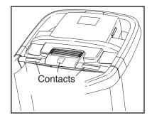
your pulse is detected, your heart rate will be shown. For the most accurate heart rate reading, continue to hold the contacts for about 15 seconds.
