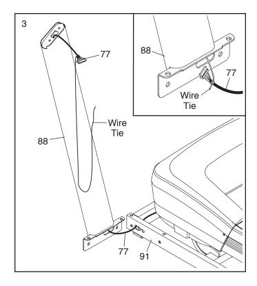
Hold the Left Upright (88) against the Base (91). Be careful not to pinch the Upright Wire (77) or the ground wire (A). Insert two 3/8" x 2 3/4" Screws (7) and two 3/8" x 1 1/4" Screws (8) with two 3/8" Star Washers (13) into the Left Upright.
