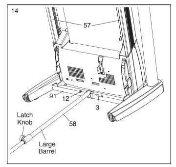
15. Attach the upper end of the Storage Latch (58) to the Frame (57) with a 3/8" x 1 3/4" Bolt (6) and a 3/8" Nut (12).
