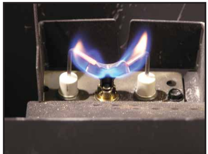
Figure 3.1 IPI Pilot Flame Patterns
