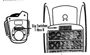
3. Slide any one or more of the switches on the receiver to the ON position. Slide the corresponding switch on the transmitter to the ON position, making sure that both devices have matching settings.
