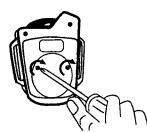
Test Caregiver Alert by pressing button on Transmitter to verify the transmitter and receiver function properly.
