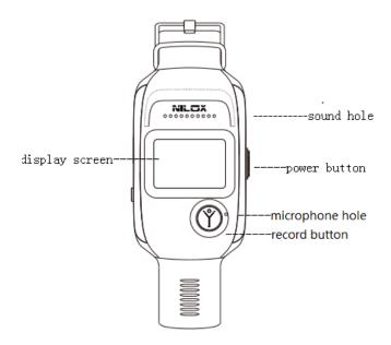
Turn on/off: Long press the power button 3 seconds (in order to ensure the safety of children, after activation watch can only be turned off through the APP remote shutdown function).
