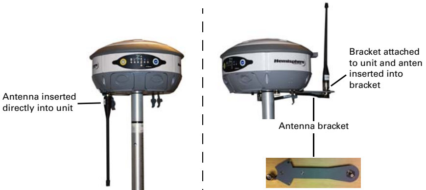
Figure 3: Antenna installation options
