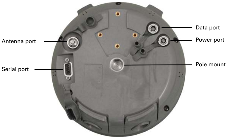
Figure 2: S320 ports and connectors
