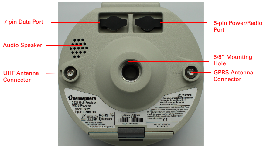
Figure 2-1: S321 ports and connectors
