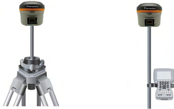
Figure 2-2: Typical base and rover setup
