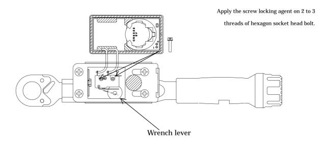
4 ) Hook the Transmitter on the Case holder of Seat, set it with an attention being paid not to bite the cord, and fix it with the set screw as firmly pushing the case.
