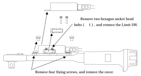
1 Since two hexagon socket head bolts(with washer) should be used later, do not lose them. Because the limit SW mounted with Torque wrench as standard has the different current capacity, do not use it.
