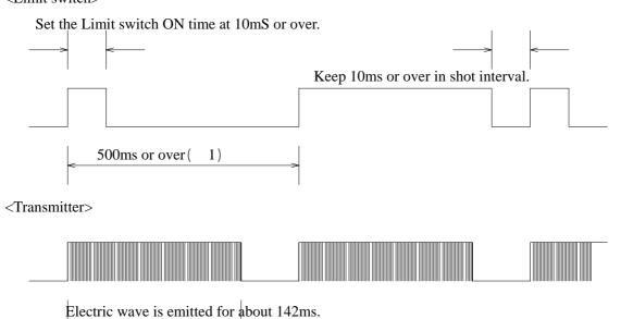
1 This interval time should be more than the double counting prevention time of Receiver.
