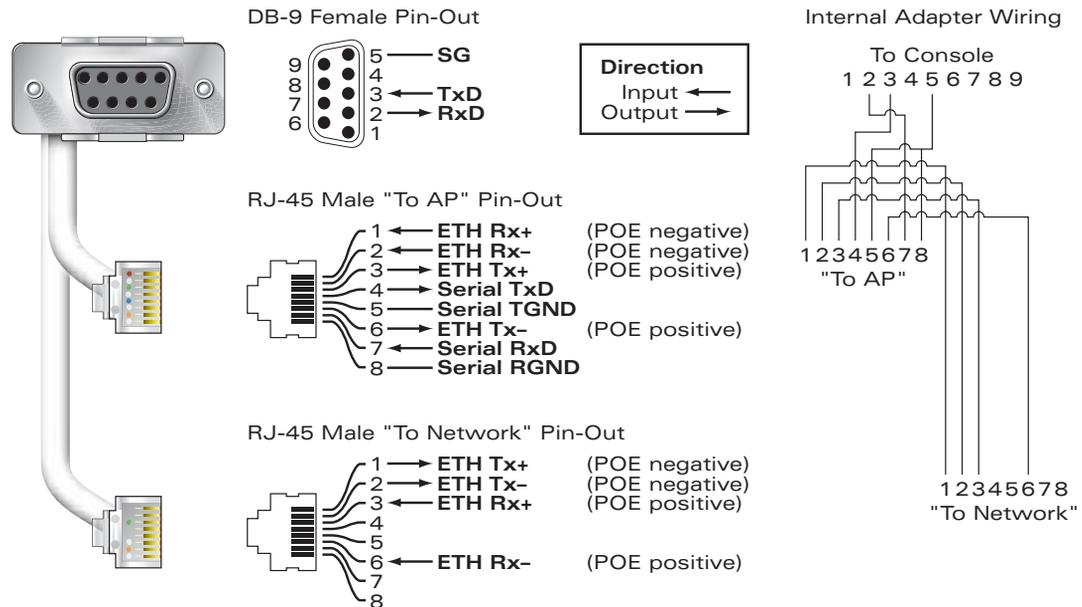
FIGURE B-2 Aruba Serial Breakout Adapter
