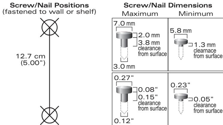
**FIGURE 2-3** Mounting Screw Specifications
