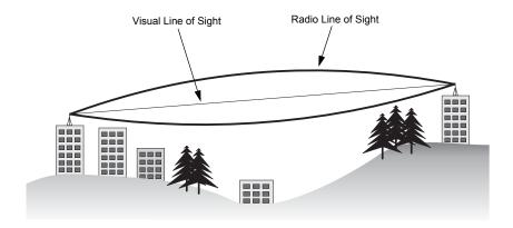
If there are obstacles in the radio path, there may still be a radio link but the quality and strength of the signal will be affected. Calculating the maximum clearance from objects on a path is important as it directly affects the decision on antenna placement and height. It is especially critical for long-distance links, where the radio signal could easily be lost.
