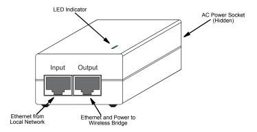
The wireless bridge does not have a power switch. It is powered on when its Ethernet port is connected to the power injector module, and the power injector module is connected to an AC power source. The power injector includes one LED indicator that turns on when AC power is applied.
