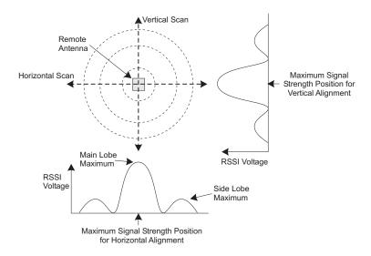
To align the antennas in the link using the RSSI output voltage, start with one antenna fixed and then perform the following procedure on the other antenna: **Note:**
