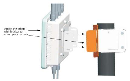
Use the included nuts to tightly secure the wireless bridge to the bracket. Be sure to take account of the antenna polarization direction; all antennas in a link must be mounted with the same polarization.
