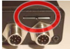
SAFEmine devices QC220 and QC24X require SIM cards to connect to the local cellular network for data transmission. The amount of data transmission can vary depending on the configurations but a data plan of XXX MB per Month has given good results.
