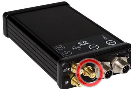
The QC24x and QC220 SAFEmine devices feature a quad-band GSM/LTE module with embedded TCP/IP stack. The module is Class 4 (2 W) for the 850/900 MHz bands and class 1 (1 W) for the 1800/1900 MHz bands.
