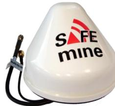
SAFEmine recommends the installation of through whole antennas (QF012 GPS/RF, QF020 GPS/GSM and QF036 GPS/RF/WiFi) for all permanent installation for its superior stability even in heavy vibration. This type of antenna is equipped with a threaded tube at the bottom to secure its position. The antenna is equipped with 15cm pigtail of coaxial cable with 50Ω wave impedance.
