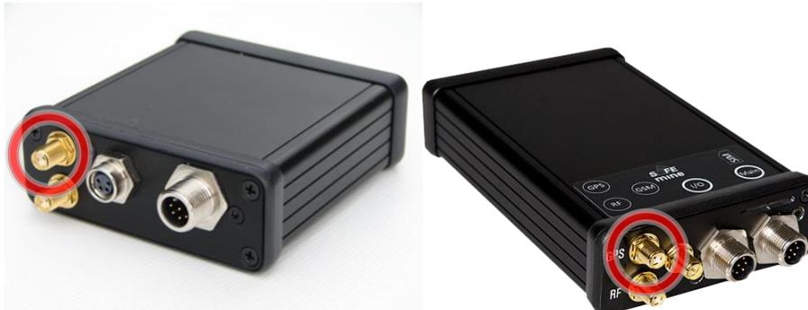
SAFEmine main units include a 50 channel GPS L1 receiver chip with SBAS (WAAS, EGNOS) capability, integrated RAIM (Receiver Autonomous Integrity Monitoring) and active multipath detection and elimination algorithms. The receiver is GALILEO ready.
