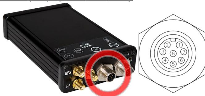
The I/O connector is an 8-pin M12 male type. The general purpose input output (GPIO) ports present on the I/O interface of the device can be used to monitor and record vehicle parameters such as: reverse gear, seatbelt clicked, bucket position, bucket load, fuel gauge, etc. The vehicle signals can be used to influence the behavior of the CAS system in order to react to different situations.
