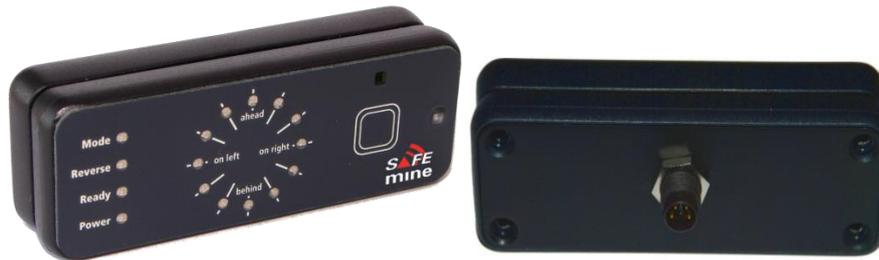
The QD200 remote display unit can be connected to all QC2xx units. The QC230 and QC235 units only require a QD221 (1.5m) or QD222 (5m) display cable extension. To connect to QC220, QC24x or QC250 units an additional QM106 display Y-cable is required.
