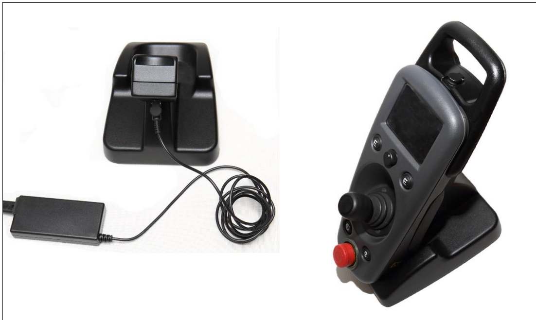
Figure 6 AC/DC Adapter plugged into the Docking Station
