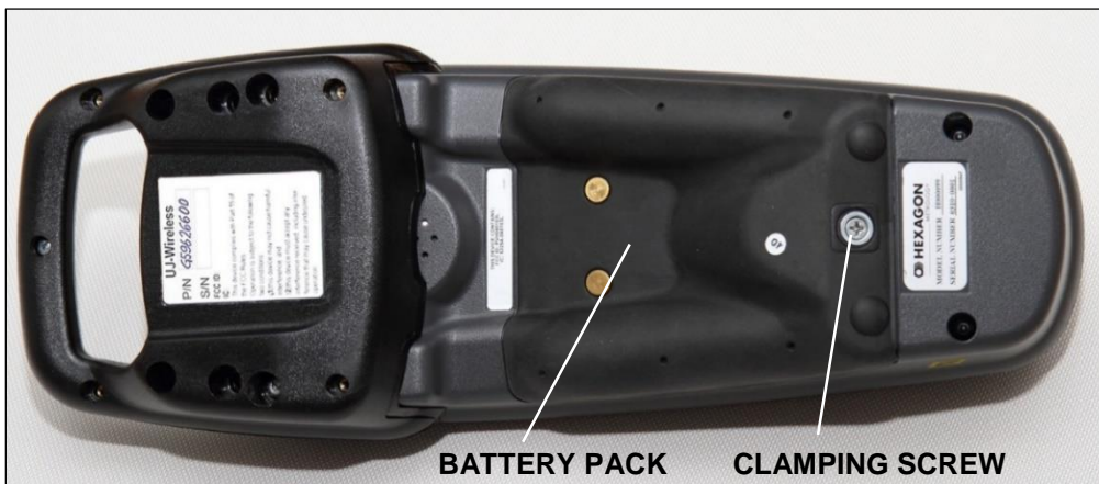
Figure 9 Battery pack in position
