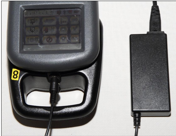
Figure 7 AC/DC Adapter plugged into the Portable Unit
