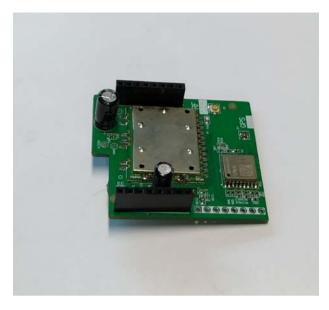
HexNet RF module is used in G3 collector of Hexing at present, with the function of wireless communication for G3 collector. RF module has the following characteristics Auto Networking, Self-maintenance, Auto Joining Network, Remote Distance. Low Power Consumption, Safe and Reliable, and so on. It's suitable for electricity meter AMR/AMI information acquisition system, resolved of local wireless the need communications.
