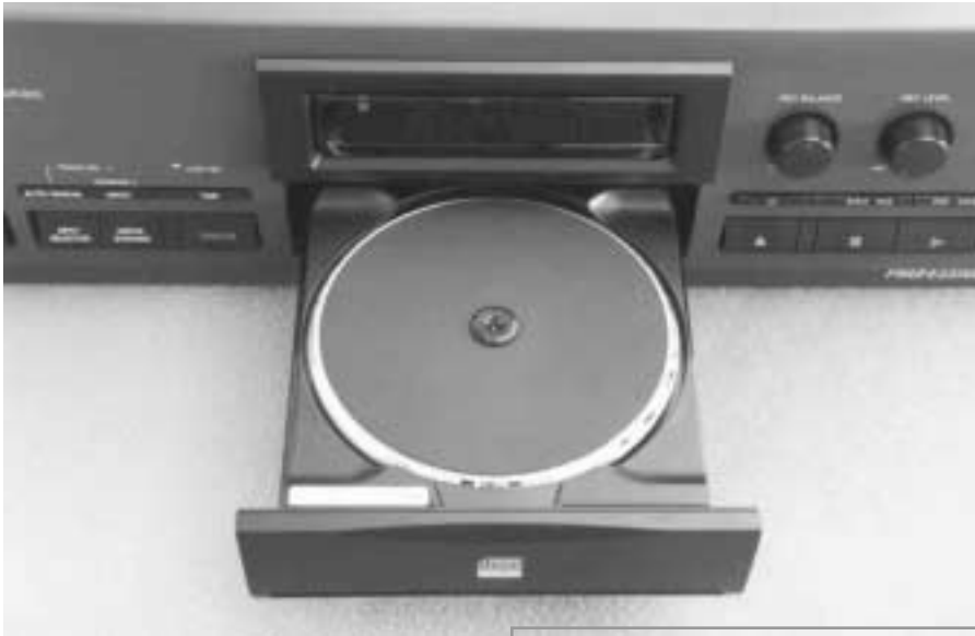
PHOTO 3: A close-up view of the Pioneer Stable-Platter mechanism used in the CDR-800. The CD must be inserted upside down, but this mechanism greatly reduces disc vibration and dust accumulation on the laser pickup.
