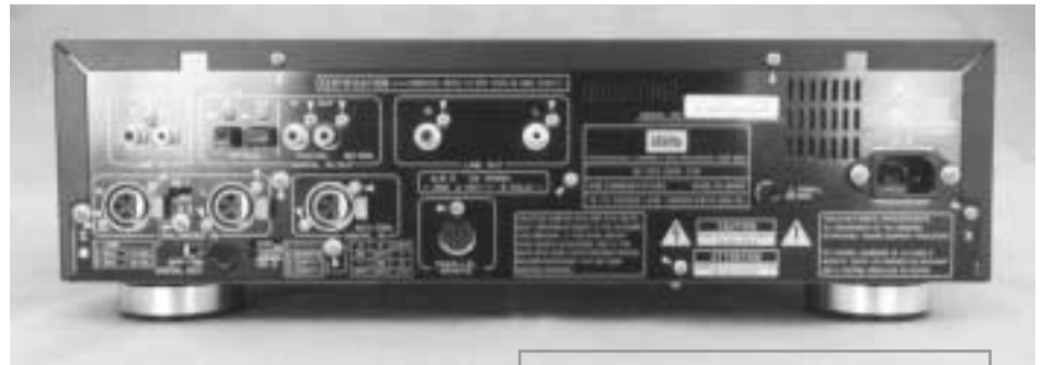
PHOTO 2: Rear panel of the CDR-800. In addition to the RCA-type analog and digital inputs, balanced XLR analog inputs and an AES/EBU balanced digital input are also provided.
