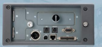
Extensive audio, synchronization, data and control connectivity includes: 6 high Word clock output on a BNC connector • Sync input (word clock, video, triqain, very low noise microphone balanced XLR-3 inputs with individual phantom level) on a BNC connector • A 5-pin LEMO socket for timecode interfacing • A 1/4" stereo jack headphone socket • A SCSI interface • An Ethernet remote control interfaces • A PS2 socket for connecting a keyboard
