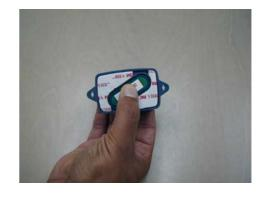
Peel the paper from the three pieces of double-sided tape: The two larger pieces (Items #3 & #4) are used for holding the DataTag to the tagged object while the smaller piece in the middle (Item #5) is used for pulling the Sensor Plate off the DataTag in order to create the TAMPER event when the DataTag is removed from the tagged object.
