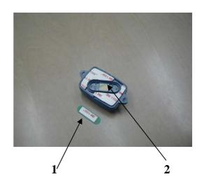
Press the sensor Tape to create the contact between the tape and the sensor Plate. Make sure the contacts at the bottom part of the plate are aligned with the pins.
