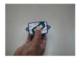
Peel the paper from the three pieces of double-sided tape: The two larger pieces (Items #3 & #4) are used for holding the DataTag to the tagged object while the smaller piece in the middle (Item #5) are used for pulling the Sensor Plate off the DataTag in order to create the TAMPER event when the DataTag is removed from the tagged object.
