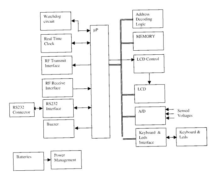
$\mu \textbf{P}$  : The  $\mu P$  (U5, Pg. 2) is a 89C52 controller with a 16MHz clock.
