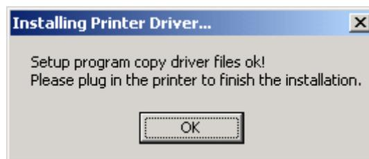
7. At this time, connect USB cable to printer and PC, then power on the machine. Windows 2000 PnP system will find the driver automatically.
