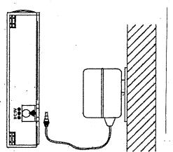
Use 2 X AA, 1.5V batteries and AC-DC adapter (AC120V, 60Hz-DC5.0V, 100mA) included.
