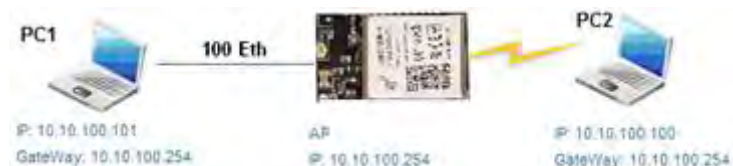
Figure 18. HF-A21-SMT Ethernet Interface Networking (As AP)
