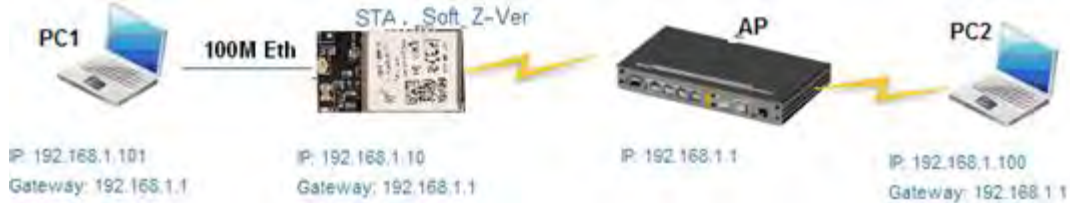
Figure 20. HF-A21-SMT Ethernet Interface Networking (As STA, Z-Ver)
