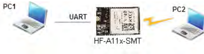
Figure 29. AP Interface Debug Connection
