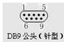
Figure 2. RS232 Pin Definition(Male/Needle Type)
