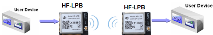
Figure 33. Transparent Serial Port Application
