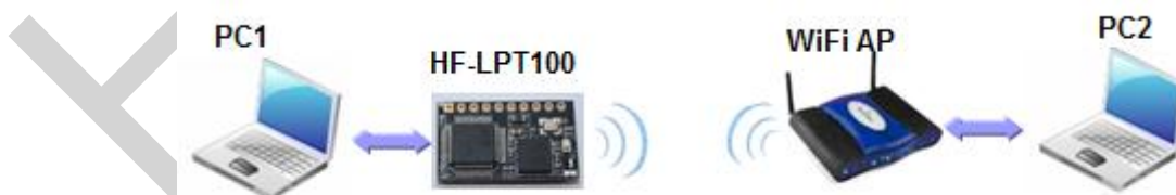
Figure 22. STA Interface Debug Connection
