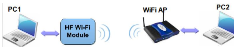
Figure 11. STA Interface Debug Connection
