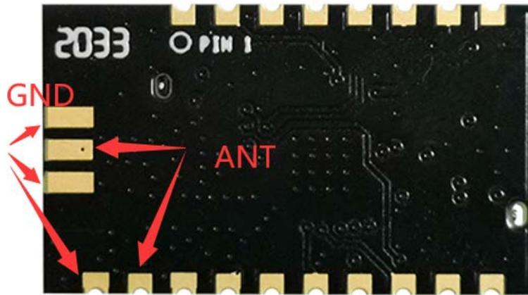
Figure 4. HF-LPT270-2 Antenna PAD Out
