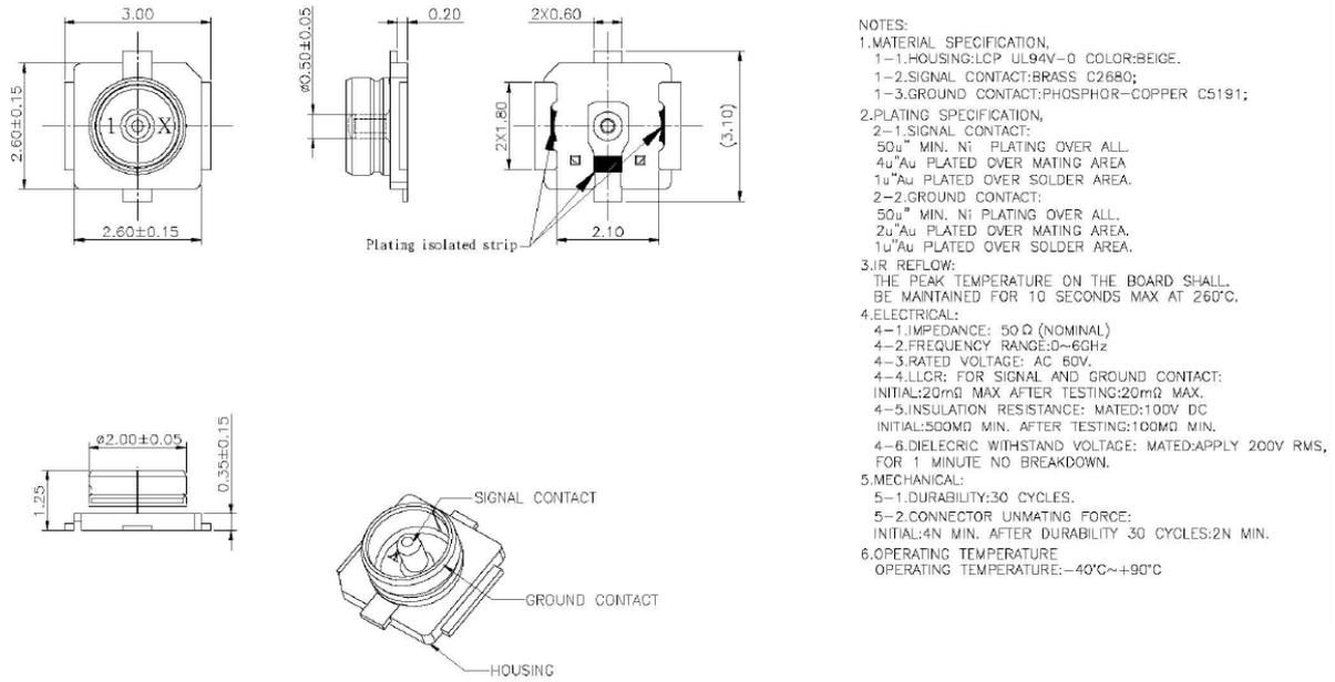
Figure 7. 1<sup>st</sup> IPEX Connector
