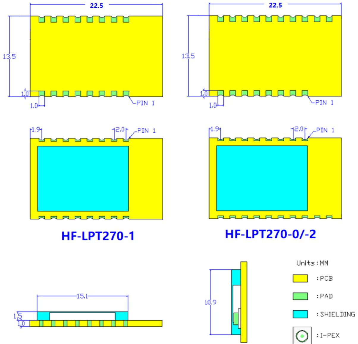
Figure 5. HF-LPT270 Mechanical Dimension
