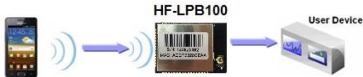
Figure 29. Wireless Control Application
