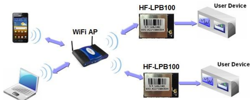
Figure 9. HF-LPB100 Basic Wireless Network Structure
