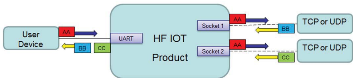
Figure 25. Multi Socket data transmission example
