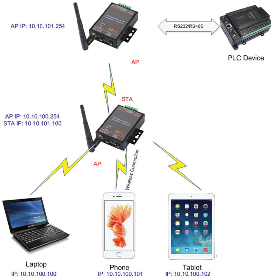
Figure 14. AP+STA Wireless Network
