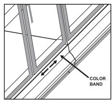
Close joints on color band by sliding the panels together. The color band can be moved left or right as required to allow adjustment.
