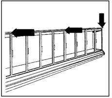
Insert exterior cornice joint at every case joint. The exterior cornice joints are shipped loose with each case
