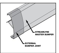
If the case has a Streamlyne front style the bumper may be shipped loose in the case. Before installing bumper on the case install the external bumper joint on the Streamlyne bumper. Simply slide the joint over the bumper for either case-to-case or case-to-end joints.
