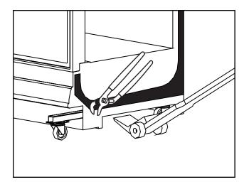
**REMOVE COTTER PIN.** Removing the casters is easy. Simply flatten and hammer out cotter pins then lift the case with "J" bar, and the casters will fall off.
