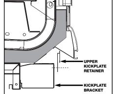
Attach the upper kickplate retainer, which is shipped loose with the case. Line up the retainer with the kickplate bracket and secure with the screws provided. The kickplate brackets are shipped loose with the ORZ and ORZH models but come installed on the ONRZ and ONRZH models.
