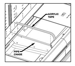
Apply acrylic tape over pipe chase seam. Tape is found with the ship loose items and acts as a watershed preventing water from settling in case joint.
