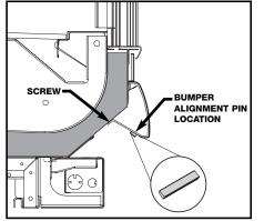
Once the Streamlyne bumper has been properly seated, attach the bumper to the tank with the screws provided. Insert the bumper alignment pin into the underside of the bumper to help align it to the bumper on the next case.
