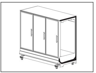
**ROLL TO LINEUP POSITION.** Casters may remain in place to move the cases to staging areas around the store, prior to final installation. When ready for final line-up, roll the case to set position, then remove casters.
