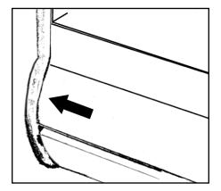
Close seam where bumper joins case end. Bumper joint closes seam that may develop if master bumper is moved away from end to close caseto-case joint seam.
