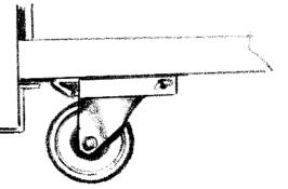
Casters not only speed up the process, but they also reduce the chance of damage from raising and lowering cases with "J" bar to place them on dollies, skates or rollers. In most situations, one or two persons can move the case with ease.
