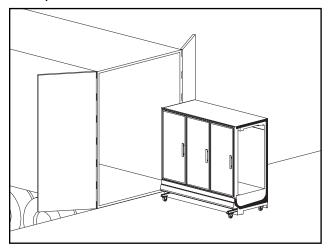
**ROLL OUT OF TRUCK.** When there is a truck - level delivery dock, cases may be rolled directly from the truck to the store floor. [CAUTION] If skid boards are required to unload cases, casters should be removed prior to sliding them down the skid; after which they can be reinstalled on case.
