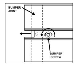
Adjust polymer master bumper joints, if required. First loosen bumper screws.
