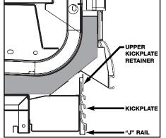
Insert top of kickplate into the upper kickplate retainer. Slide the kickplate up into retainer then down on the "J" rail.
