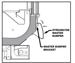
Place the hook of the Streamlyne bumper on the lip of the master bumper bracket and rotate the bumper down while pushing it in. Once the top edge of the bumper has slipped under the color band make sure it is pushed in as far as it will go.
