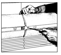
Slide bumper joint to the center of the joint between the two cases. Use screw driver in hole provided.
