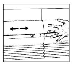
Slide master bumper left or right to close seam as required. Bumper joint neatly finishes any gap that may remain.
