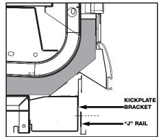
Attach the "J" rail, which is shipped loose with the case. Line up the rail with the kickplate bracket and secure with the screws provided.
