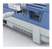
c. Push the cord connector into the foot switch port until the connector automatically makes a 1/4 turn and you hear a click sound.
