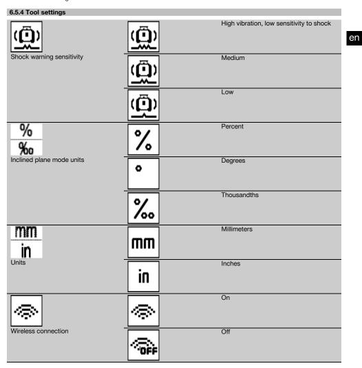
Settings that affect the rotating laser only become effective when the rotating laser is switched on and a wireless connection has been established. Pressing the "Back" key  $\mathfrak D$  takes you back to the main menu.
