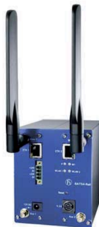
Figure 12: Connections for external antennas on BAT54-Rail
