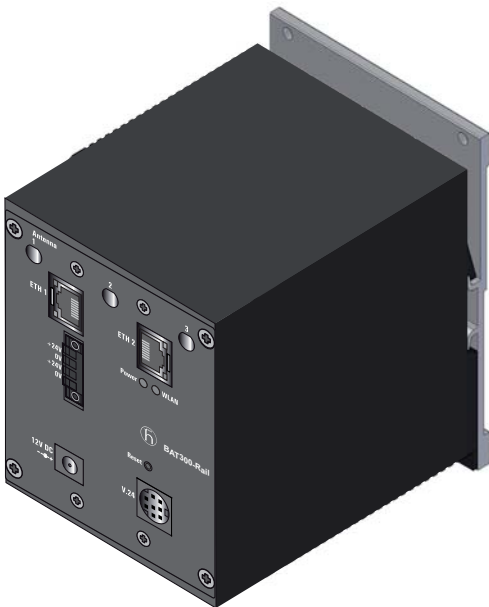
Figure 7: BAT-Rail, wall mounting
