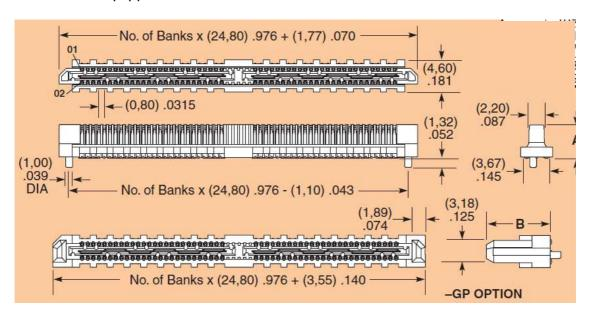
The host equipment has to be equipped with Samtec connector QRF8-026-05.0-L-D-A-GP
