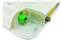
3.) Insert the fiber into the cover slot and slide the cover back onto the 72xx unit.
