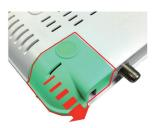
2.) With the fiber connector exposed, remove the dust plug, clean the fiber ends and terminate the SC equipped fiber.
