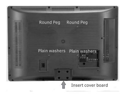
5. Meet the mounting holes of the back panel with the fixture disks in the brackets and fix the TV to the wall-mounting bracket. Be cautious of the TV from falling.
