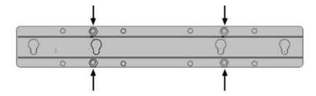
3.Lay the TV on a plane table which could bear enough weight, and cover the surface of the table with soft cloth to avoid damage to LCD panel. Remove the four bolts fixing the stand and remove the stand from TV.
