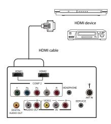
**Note:** To connect a DVI device, use a DVI to HDMI adapter cable to connect to the **HDMI** jack on the TV, then connect an audio cable to the **PC AUDIO** jack on the back of the TV.
