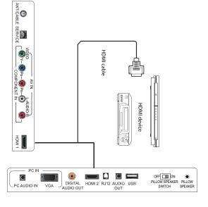
**Note:** To connect a DVI device, use a DVI to HDMI adapter cable to connect to the **HDMI** jack on the TV, then connect an audio cable to the **PC AUDIO** jack on the back of the TV.
