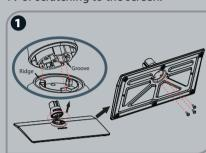
Align the front of the stand column with the front of the base, then insert the stand column into the base making sure that the groove in the stand column aligns with the ridge in the base. Secure the stand column to the base with 3 Screws A (M5 x 12)
