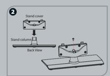
Align the stand cover with the stand column, then secure the stand cover to the stand column with 1 Screw A (M5 x 12). Make sure that the bottom of the stand cover is flush against the top of the stand column.
