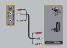
Connect the composite video and audio output jacks of your legacy A/V equipment, such as a VCR.
