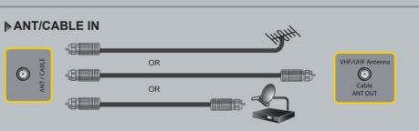
Connect to a broadcast antenna or cable TV.
