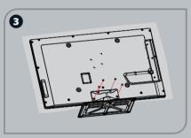
Secure the stand to the TV with the 4 Screws A (M5 x 12).
