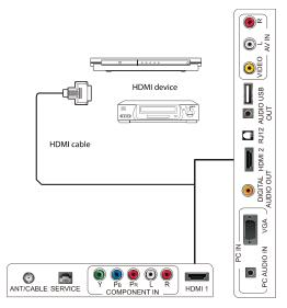
**Note:** To connect a DVI device, use a DVI to HDMI adapter cable to connect to the **HDMI** jack on the TV, then connect an audio cable to the **PC AUDIO** jack on the back of the TV.
