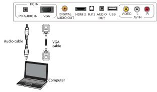
3 Connect one end of an audio cable with a stereo mini-plug (not included) to the PC AUDIO jack on the side of the TV, then connect the other end of the cable to the AUDIO OUT jack on the computer.
