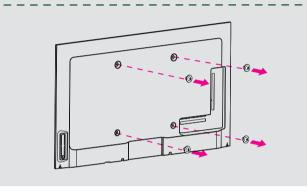
cushioned space, remove the original screws in the bracket holes on the TV back.
