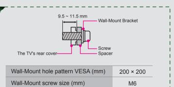
Follow instructions provided with the Wall-Mount bracket. If you are not sure of your ability to do complete the installation, contact a professional installer or service technician for assistance. The manufacturer is not responsible for any damages or injuries that occur due to mishandling or incorrect assembly. The selected screws are 9.5 ~ 11.5 mm in length when measured from the attaching surface of the TV's rear cover. The diameter and length of the screws differ depending on
