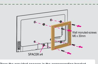
holes. Attach purchased bracket (1.5mm to 2.5mm thickness) on the TV with 4 screws which are in the accessories bag. Follow instructions provided with the wall-mount bracket.
