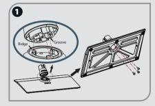
Align the front of the stand column with the front of the base, then insert the stand column into the base making sure that the groove in the stand column aligns with the ridge in the base. Secure the stand column to the base with 3 Screws(M5 x 12).
