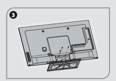
Secure the stand to the TV with the 4 Screws (M5 x 12).
