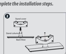
Align the stand cover with the stand column, then secure the stand cover to the stand column with 1 Screw (M5 x 12). Make sure that the bottom of the stand cover is flush against the top of the stand column.
