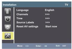
3 Press ▲ or ▼ to highlight an option, then press **ENTER** or ► to access the option, and press ⋖ or ► to adjust the option. You can select:
