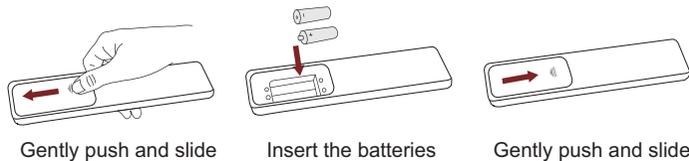
2. Insert two AAA size batteries. Make sure to match the (+) and (-) ends of the batteries with the (+) and (-) ends indicated in the battery compartment.
