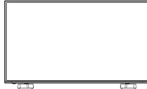
2. Place the legs into the bottom slots of the TV, insert and tighten the screws (found in the accessories bag) in the circled area with the screwdriver (not provided).
