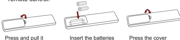
2. Insert two AAA size batteries. Make sure to match the (+) and (-) ends of the batteries with the (+) and (-) ends indicated in the battery compartment.
