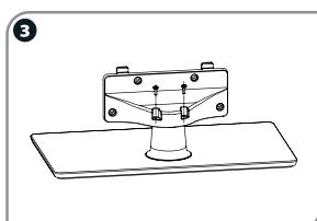
Secure the stand cover to the stand column vertically with the 2 screws (M4×12) provided. (For 55": (M5×12))
