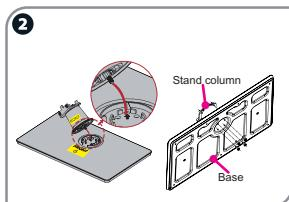
Insert the stand column into the base plate, aligning the ridge on the column with the groove in the base plate. Making sure the FRONT of stand column matched with the FRONT of base plate. Secure the stand column to the base plate with the 4 Screws (M4 × 12). (For 55": (M5×12))
