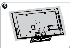
Secure the stand cover to the TV with the 4 screws (M5×12) provided.
