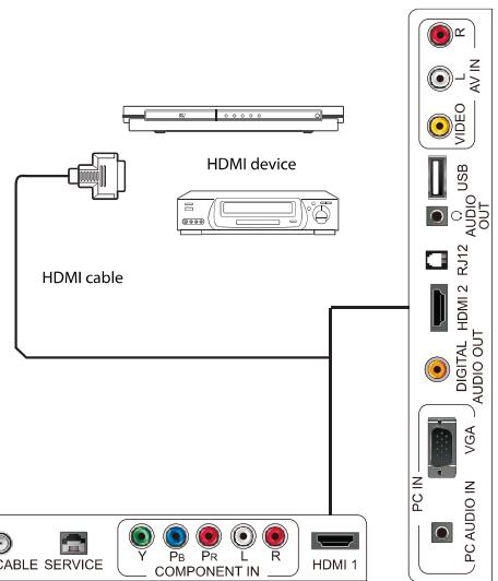
**Note:** To connect a DVI device, use a DVI to HDMI adapter cable to connect to the HDMI jack on the TV, then connect an audio cable to the PC AUDIO IN jack on the back of the TV.
