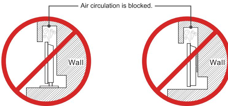
Inadequate air circulation can lead to overheating of the TV and may cause damage to your TV or cause a fire.
