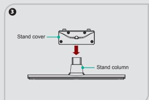
Align the stand cover with the stand column. Make sure that the bottom of the stand cover is flush against the top of the stand column.
