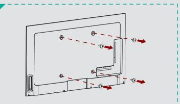
Make sure the TV is laid face-down on a clean, safe, and cushioned space, remove the original screws in the bracket holes on the TV back. NOTE: These 4 screws which got from back cover mount hole could not
