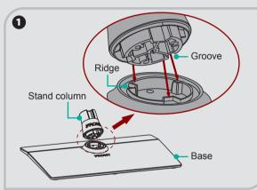
Align the front of the stand column with the front of the base, then insert the stand column into the base making sure that the groove in the stand column aligns with the ridge in the base.
