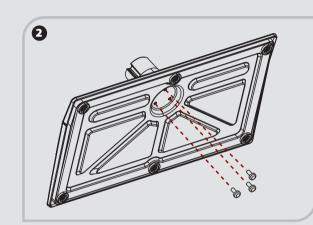
Secure the stand column to the base with 3 screws
