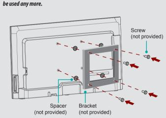
Place the spacers (not provided) in the corresponding bracket Follow the instructions provided with the wall-mount bracket to attach the bracket on the TV.
