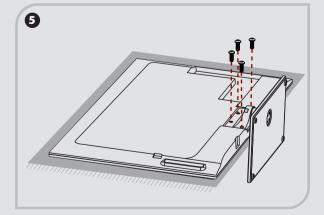
After pre-installing the stand, secure the stand to the TV with the 4 screws (M5×12).
