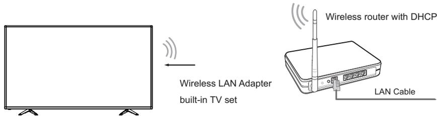
The TV can directly receive network signals via wireless router
